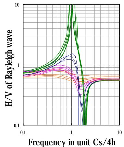
Figure 4. H/V of Rayleigh wave for two layered ground
