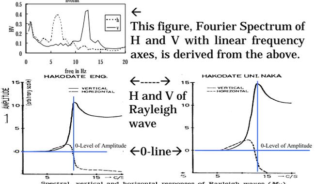
Fig. 7. Underground structure. Observed and theoretical ratio of the horizontal component ( $\omega_h$ ) to the vertical component ( $\omega_v$ ) of Rayleigh wave ( $M_R$ ).
